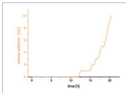
Figure 6: Added amount of antifoam (Antifoam 204, Sigma) solution during the *Escherichia Coli* cultivation
