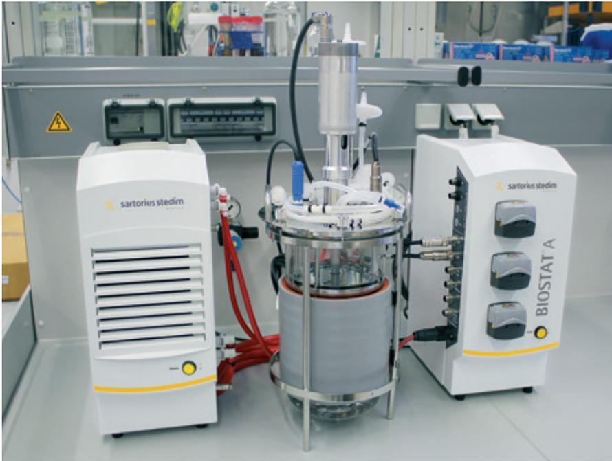
Figure 1: BIostat® A setup for the *Escherichia coli* high cell density fermentation experiment
